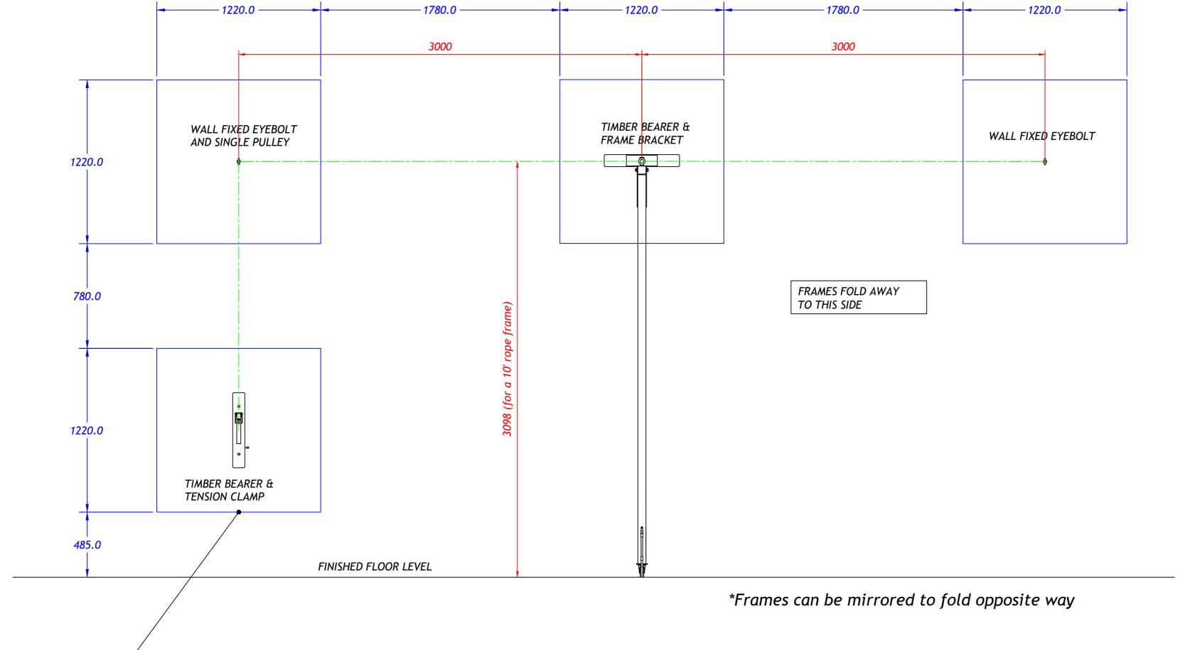
4no blue rectangles indicate plywood to walls to accommodate frame fixings. Minimum 18mm thk pattress can be surface mounted or between studs.
