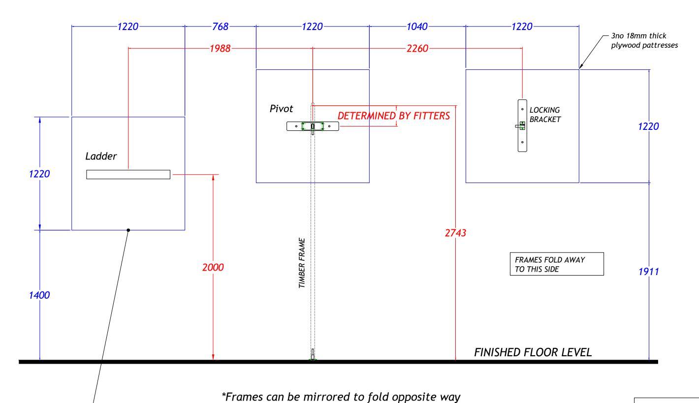
3no blue rectangles indicate plywood to walls to accommodate frame fixings. Minimum 18mm thk pattress can be surface mounted or between studs.
