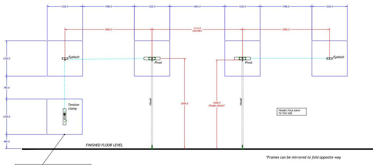
5no blue rectangles indicate plywood to walls to accommodate frame fixings. Minimum 18mm thk pattress can be surface mounted or between studs.
