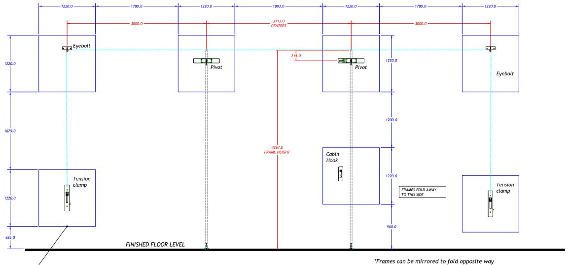
7no blue rectangles indicate plywood to walls to accommodate frame fixings. Minimum 18mm thk pattress can be surface mounted or between studs.
