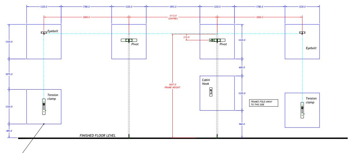
7no blue rectangles indicate plywood to walls to accommodate frame fixings. Minimum 18mm thk pattress can be surface mounted or between studs. \*Frames can be mirrored to fold opposite way
