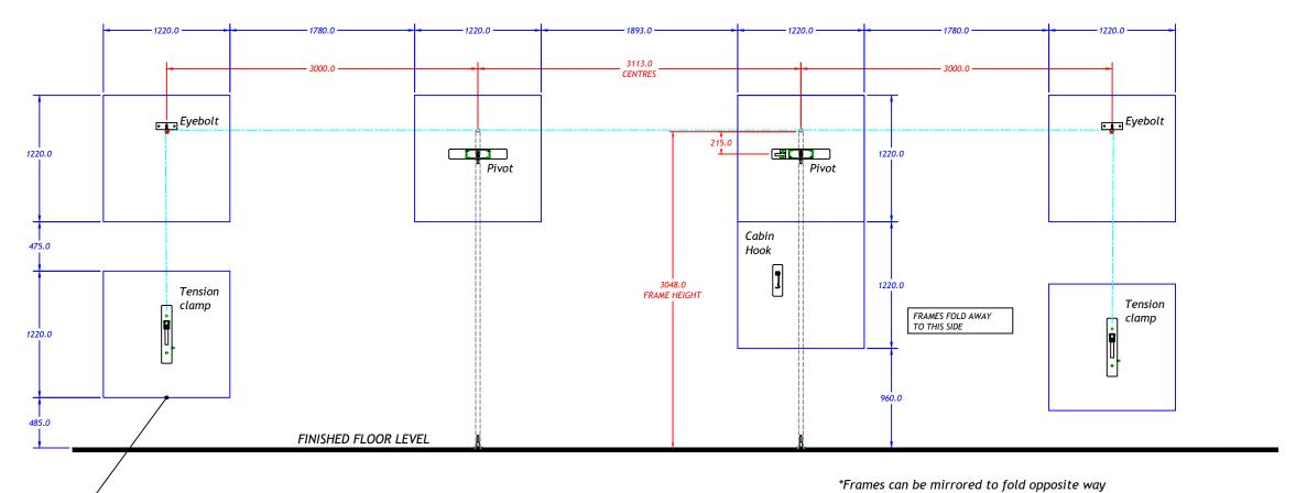
7no blue rectangles indicate plywood to walls to accommodate frame fixings. Minimum 18mm thk pattress can be surface mounted or between studs.
